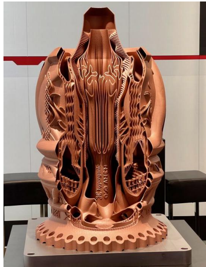
Figure 1. The 3D printed copper Aerospike rocket engine [Source: Fabbaloo ]
